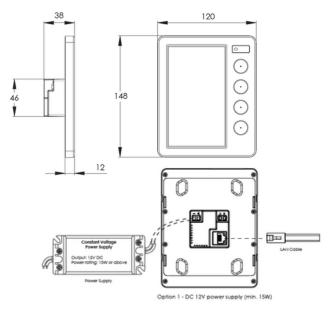
Powered by either POE or a low voltage power supply for simple installation. Fits into a standard single-gang wall plate mount and provided with metal mounting bracket and template for precise mounting.
