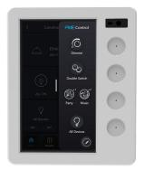
Pull out menu acts as a reminder of button functions and fast multifunction button reconfiguration tool.
