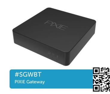
The PIXIE Gateway works with the PIXIE system and needs the free PIXIE Plus app. This device is a bridge between the internet and the PIXIE Bluetooth mesh inside the home, introducing additional features and functionality such as out of home control and voice control capabilities. Comes with Bluetooth Mesh and Wireless (2.4GHz connectivity.
